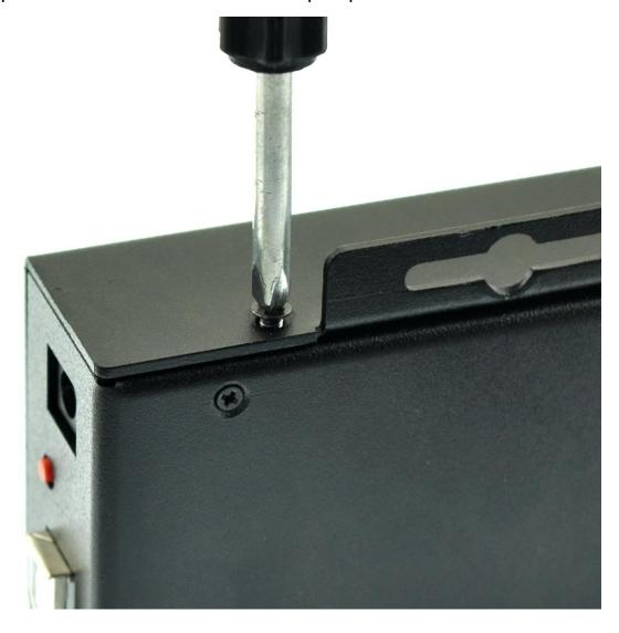
7, Install DIN rail adapter bracket with a phillips screwdriver. if you don't need DIN rail mount, you don't have to install it.
