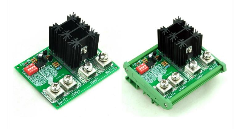
To protect electronics from damaging low voltages and prevent a deep discharge of a battery during an extended power outage, the LVD module will automatically disconnect the battery when the voltage falls below the user adjustable cutoff voltage. When power is restored the Smart Switch will automatically reconnect the battery. thereby protecting the battery from total discharge (helping to prolong the life of the battery).
