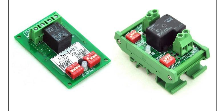
To protect electronics from damaging low voltages and prevent a deep discharge of a battery during an extended power outage, the LVD module will automatically disconnect the battery when the voltage falls below the user adjustable cutoff voltage. When power is restored the Smart Switch will automatically reconnect the battery, thereby protecting the battery from total discharge (helping to prolong the life of the battery).
