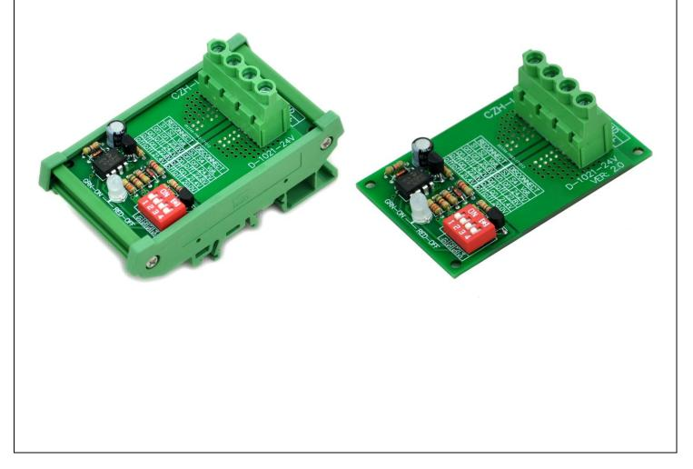
To protect electronics from damaging low voltages and prevent a deep discharge of a battery during an extended power outage, the LVD module will automatically disconnect the battery when the voltage falls below the user adjustable cutoff voltage. When power is restored the Smart Switch will automatically reconnect the battery. thereby protecting the battery from total discharge (helping to prolong the life of the battery).
