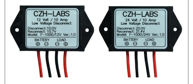
To protect electronics from damaging low voltages and prevent a deep discharge of a battery during an extended power outage, the LVD module will automatically disconnect the battery when the voltage falls below the cutoff voltage. When power is restored the Smart Switch will automatically reconnect the battery. thereby protecting the battery from total discharge (helping to prolong the life of the battery).
