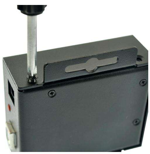
7, Install DIN rail adapter bracket with a phillips screwdriver. if you don't need DIN rail mount, you don't have to install it.
