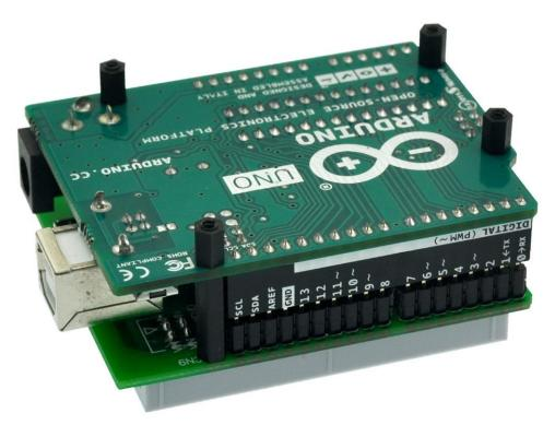
4, Install bottom cover and M2x6mm screws with a small phillips screwdriver.
